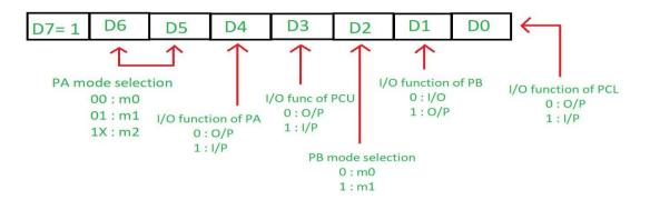
The most significant bit (**D7**) is 1 for the I/O mode and 0 for the BSR mode. **D6 & D5**It is used to set the port A mode.
