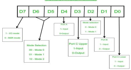
If the most significant bit of control word or D7 is 1 then 8255 works in I/O mode else, if it's value is 0 it works in BSR mode.
