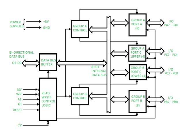
It consists of 40 pins and operates in +5V regulated power supply. Port C is further divided into two 4-bit ports i.e. port C lower and port C upper and port C can work in either BSR (bit set rest) mode or in mode 0 of input-output mode of 8255. Port B can work in either mode or in mode 1 of input-output mode. Port A can work either in mode 0, mode 1 or mode 2 of input-output mode.
